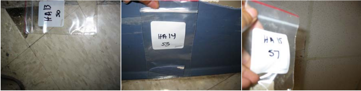
HA 13: Throughout building, 1x1 beige floor tile with blue specks HA 14: Throughout building, blue mopboard HA 15: Throughout building, 2x4 white lay-in ceiling tile fissured
