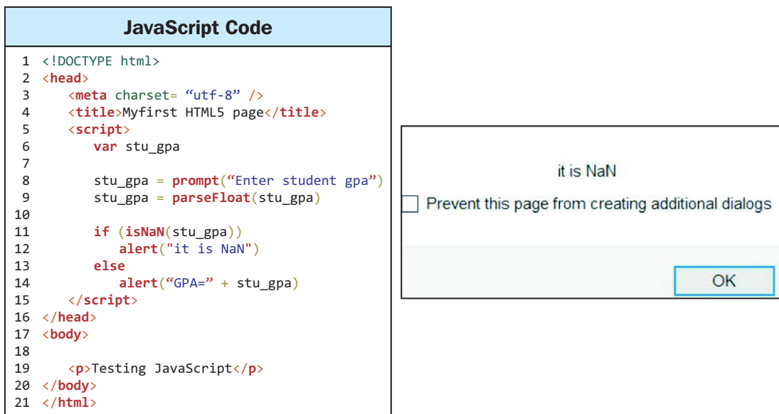
FIGURE 17. This example shows the remonstrating use of the isNaN function. When a user enters a value via the prompt function, the value is converted into a number using the parseFloat or the parstInt function. However, if the user enters a non-numeric value, which cannot be converted by the parseFloat or parseInt functions, NaN is placed in the variable that was to be populated via the prompt statement.
