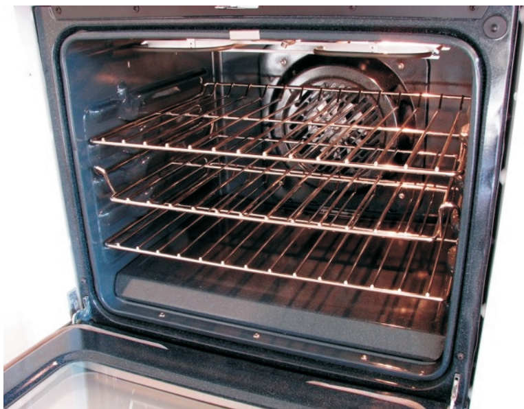
FIGURE 2. Convection ovens cause hot air to circulate around the foods (horizontally), causing the food to cook and brown more evenly. Notice the fan at the back of this oven. Convection ovens cook food 25 percent faster at a temperature 25 percent lower than a conventional oven.
