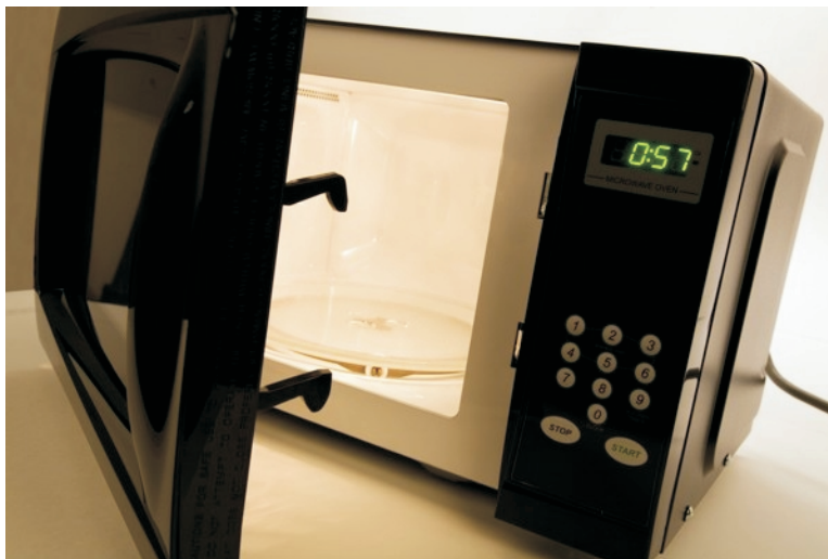
FIGURE 3. Notice that the clips on the microwave oven door ensure that the door cannot accidentally open while the oven is in operation.
