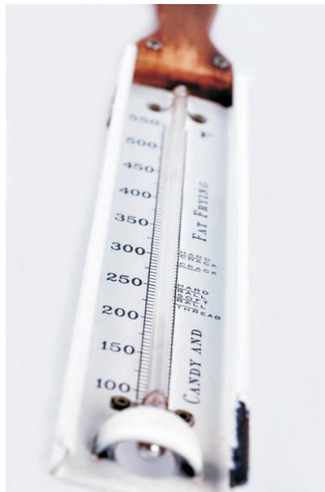
FIGURE 1. This thermometer is for measuring candy and deep-fry temperatures. Notice that it measures temperatures above 500°F.
