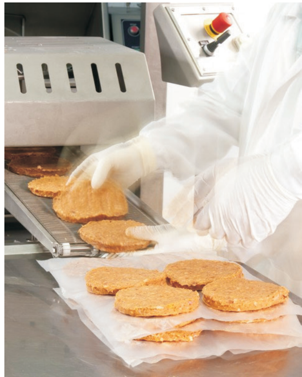
FIGURE 5. Notice the red emergency stop button on this hamburger machine.
