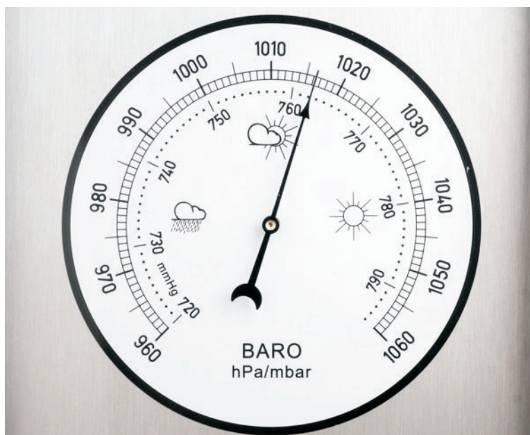
FIGURE 6. On this gauge, notice the correlation between the barometric pressure numbers and the predicted weather.
