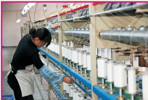
In 1828, American John Thorp invented the spinning machine used today. Hundreds of spindles are mounted vertically to simultaneously produce large quantities of yarn.
