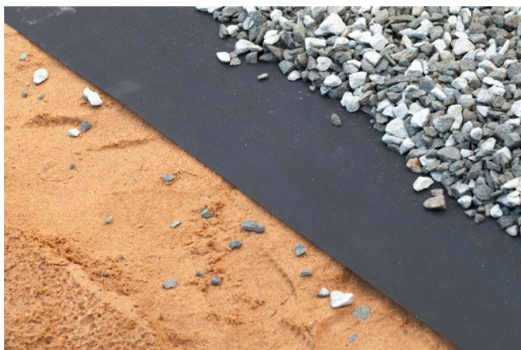
FIGURE 1. The roadway fabric pictured is a geotextile that is placed between gravel and sand prior to a road surface application. The awnings shown are in a downtown area of Madrid, Spain, where preparation is underway for a summer festival.
