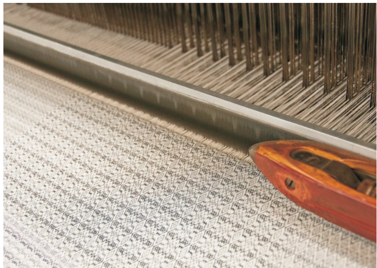
FIGURE 6. This is a sample of white-on-white fabric on a doobby weaving loom.
