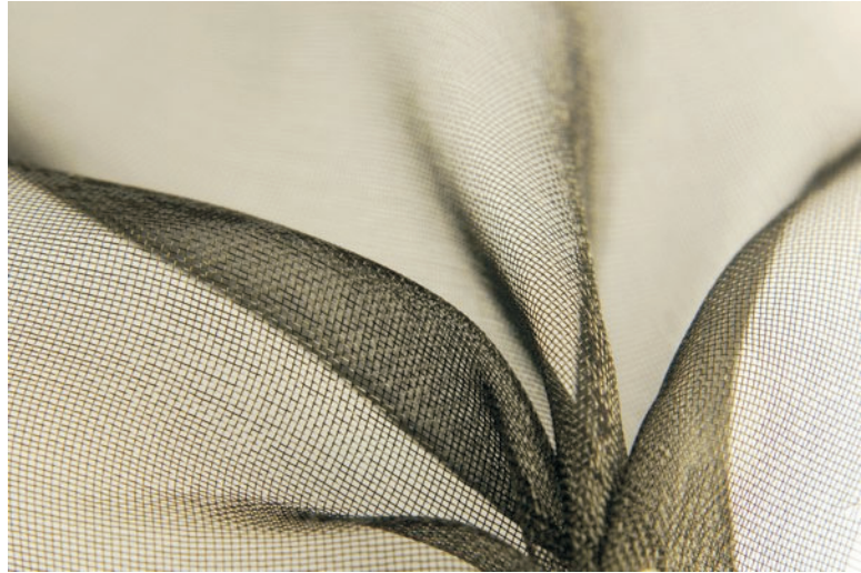
FIGURE 2. This plain-weave organza fabric illustrates how one woof yarn is woven over and under one warp yarn. Plain organza fabrics are used for decorative bows and gift bags, as well as garments and window covers.
