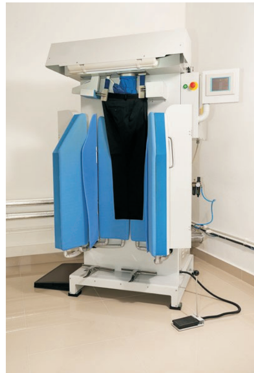
FIGURE 2. A pant presser is a piece of equipment used to take the wrinkles out of pants and put a crease in them. The pant presser has two main pieces: a heating pad and a pressing plate with stretcher bars.
