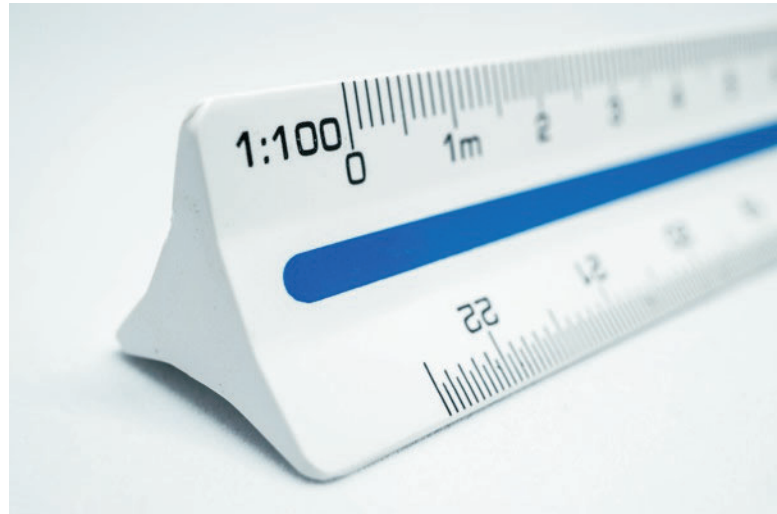
FIGURE 2. A scale-ruler is a measurement tool with a range of calibrated scales (ratios) for drawing and measuring from reduced scale drawings, such as blueprints and floor plans.
