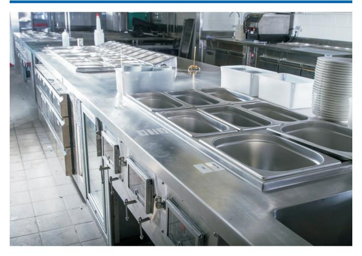
The sandwich station (in the foreground) has one-half and one-third hotel pan inserts to load meats, cheeses, vegetables, and garnishes. These refrigerated units have extra storage below the working surface with back-up materials, a ledge for prep in front, and a space for carryout and pickup by the front-of-the-house servers.
