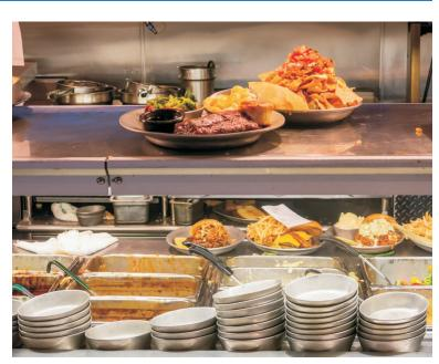
◆ This chef has various sizes of hotel pans and a bain-marie at his disposal. A hotel pan is a standard-sized stainless steel pan designed to fit perfectly in openings or wells on steam tables or refrigerated tables. A bainmarie is a round-in-shape cylindrical vessel that holds finished soups and sauces that is placed inside another container filled with hot water or hot air.
