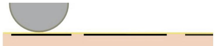
STEP 5. The paper is removed and the print has been transferred from the plate to the paper.
