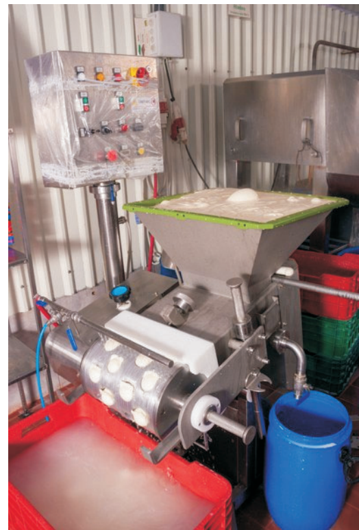
FIGURE 6. Food technologists work at small pilot plants or do a test production in a full-scale manufacturing facility. This pilot plant is processing fresh mozzarella cheese.
