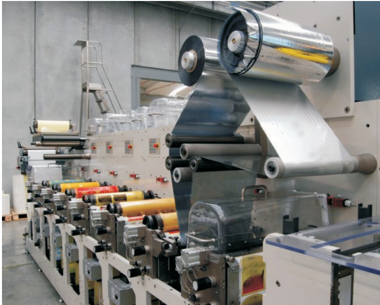
FIGURE 3. A Flexo press is used to print labels for all types of packaging. “Flexography” is another term for “surface printing.” The press can print on plastic, metal, paper, and cellophane.
