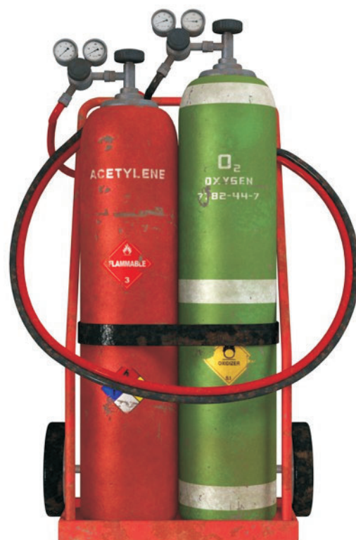
FIGURE 1. These cylinders are secured in a safe upright position on an oxyacetylene welding cart.
