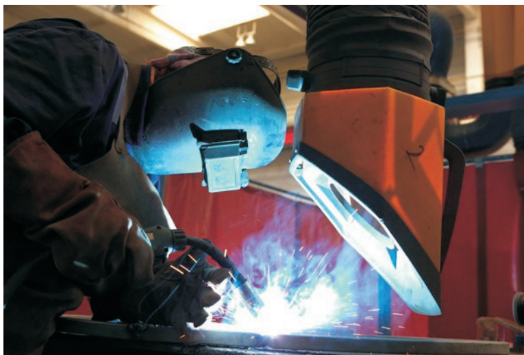
FIGURE 1. This man is welding using proper safety gear and ventilation.
