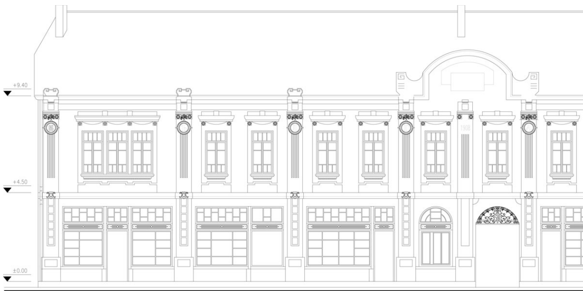
FIGURE 2. Several line weights are used to designate features of this building elevation drawing.
