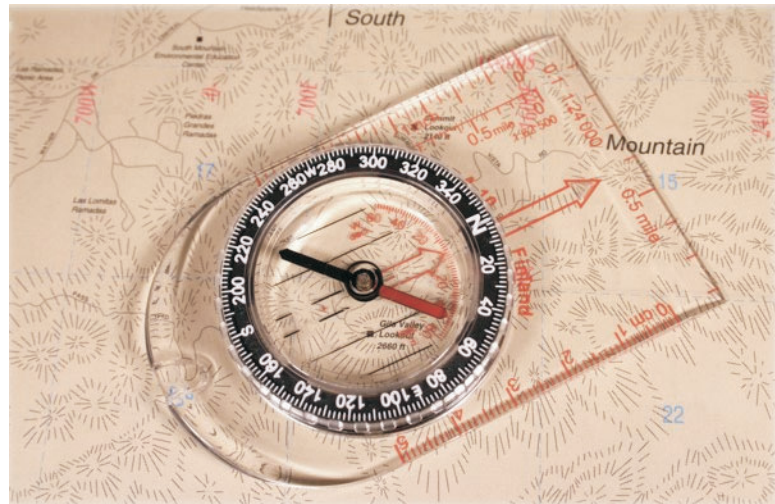
FIGURE 4. Compass bearings are used to designate the direction of an object on civil engineering drawings.
