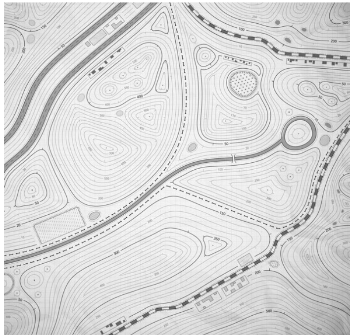
FIGURE 3. Contour lines allow the civil engineer and construction crew to see changes in elevation on a flat two-dimensional drawing. This image is a topographic drawing with contour lines.
