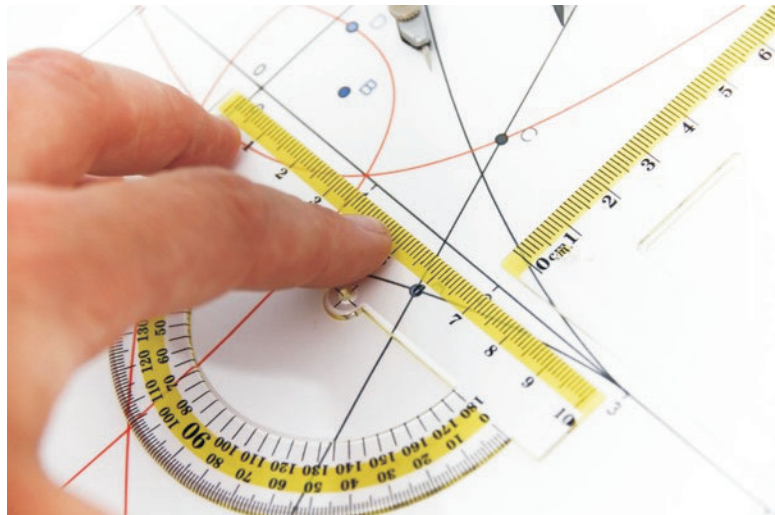
FIGURE 6. Use of a protractor is necessary to create lines at specific angles. Protractors are used in combination with a straightedge, T-square, or triangle to draw lines at any direction.
