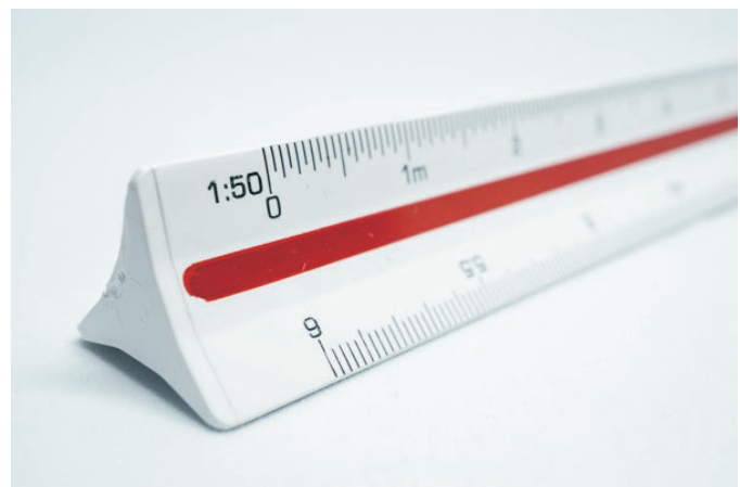
FIGURE 3. A scale ruler is used to reduce or enlarge a technical drawing.
