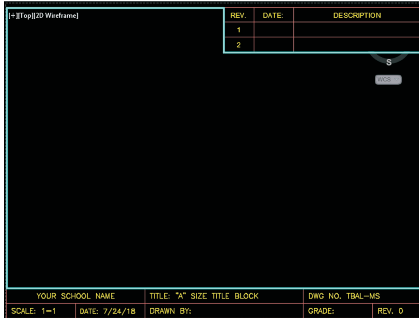
FIGURE 11. AutoCAD’s polygonal viewport with model space activated is pictured here. (AutoCAD screen shot reprinted with the permission of Autodesk, Inc.)
