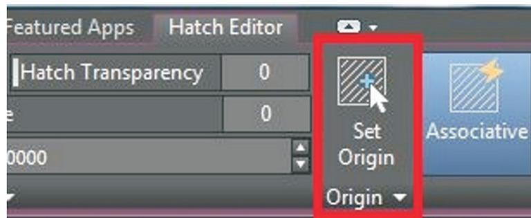
FIGURE 9. This is the location of AutoCAD's 'specify new origin menu.' (AutoCAD screen shot reprinted with the permission of Autodesk, Inc.)
