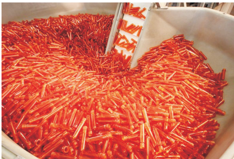
FIGURE 2. Plastics blanks are being prepared to be used to manufacture bottles at a plant.
