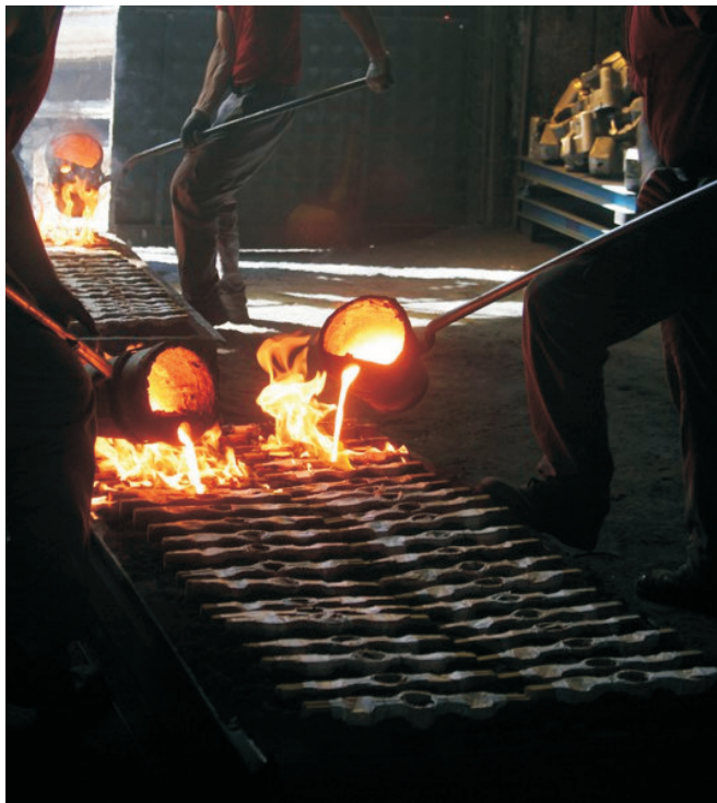
FIGURE 1. Metals are being put through the casting process. Notice the high temperatures required.
