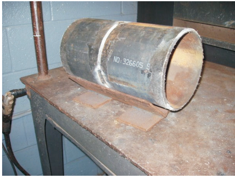
FIGURE 2. This is a pipe 1G welding position. (Image provided by David Zielinski, http://www.gowelding.org )
