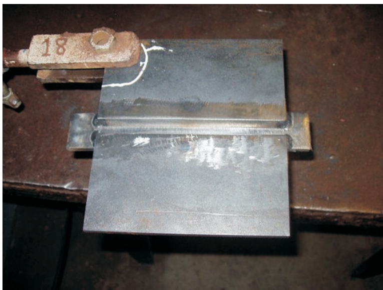
FIGURE 1. This is a structural 1G welding position. (Image provided by David Zielinski, http://www.gowelding.org )
