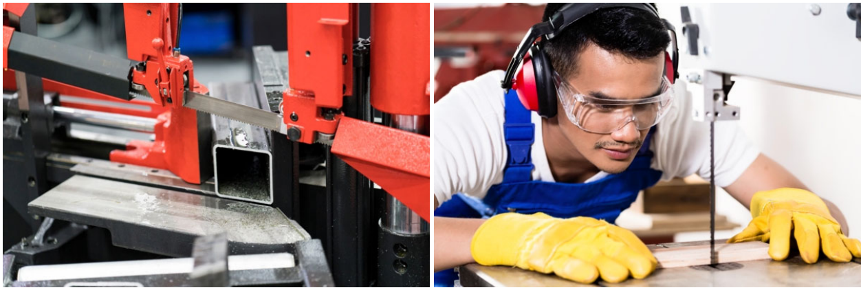
FIGURE 4. There are several different types of band saws. Some are used for small detailed pieces of wood, some for larger wood stock, and some are used for metal. It is always important that you use the correct tool for the material and job.
