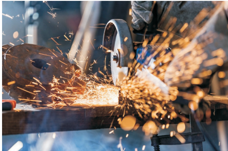
FIGURE 6. Grinding machines have several moving parts and can produce a lot of debris and sparks, so it is important to follow all steps and make sure you wear proper protection.
