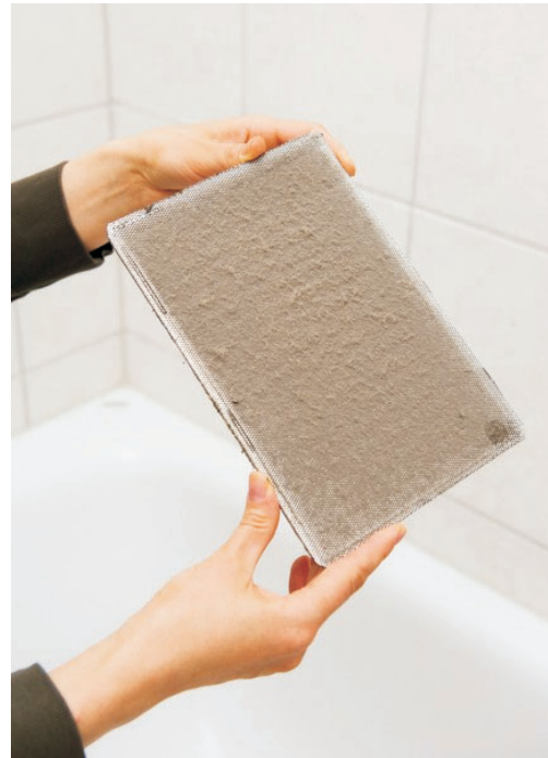
FIGURE 3. Dirt and mold can impede airflow.
