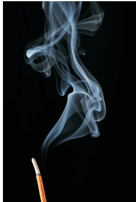
FIGURE 2. A smoke stick can show air movement.
