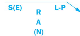
(b) Location of dimensions when weld symbol is on arrow side of reference line
