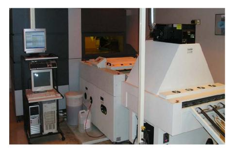
This process is accurate and timely can will provide up to 100 plates or "signatures" per hour. A signature is one 11" x 17" sheet which consists of four  $8\frac{1}{2}$ " x 11" images. In the case of Illinois largest booklet, the third grade booklet, the plate process took just over one hour per form for the one hundred pages.
